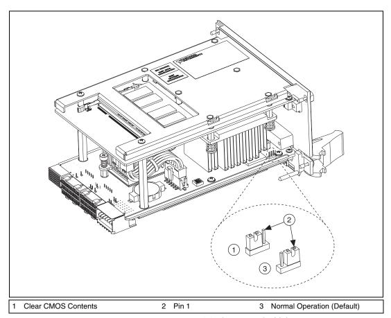
Figure 2-3. Clearing the CMOS Contents
